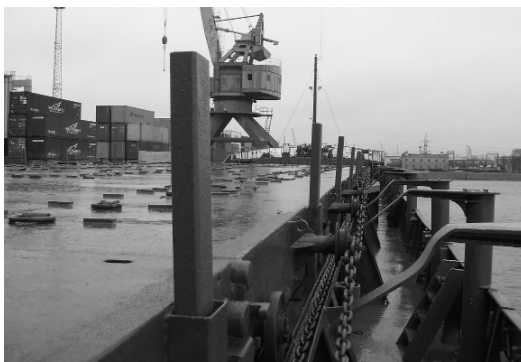
Figure 6.7. Example of uprights for bottom blocking
